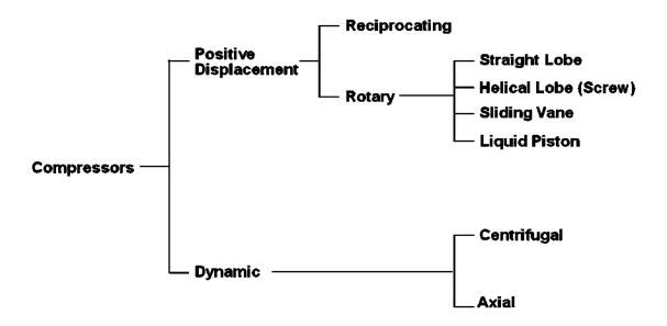
Reciprocating compressors compress gas by a piston moving back and forth within a cylinder. It is the most common type of positive displacement compressor found in an industrial pneumatic system.
