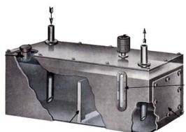
Baffles are an important component in a hydraulic reservoir. They allow the fluid time to cool, de-aerate, and to settle out water and dirt. A good rule of thumb to use for residence time in a reservoir is 2 to 3 times the pump output. If the system is highly contaminated, residence time may be 10 times the GPM (gallons/minute) of the pump.
